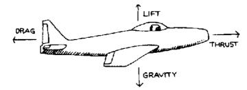
There is still another way most real aeroplanes and some paper aeroplanes use their wings to increase lift. The top-side as well as the bottom side of the wing can help to give the plane lift.
