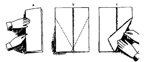
Fold the paper in half lengthwise (a). Make sure you crease all the folds sharply with your thumbnail. Open the paper. Fold one corner up (c) along the dotted line shown in drawing b. Note that the point you form at the bottom of the paper should be slightly to the left of the midline.
