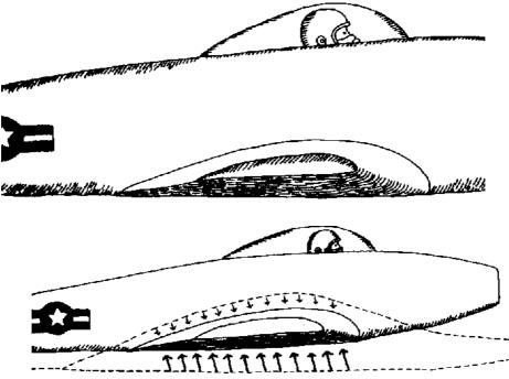
Thrust makes the aeroplane move through the air. The shape of the wing forces the air to move over and under it. The air moving over the top reaches the back of the wing at the same time as the air moving across the bottom of the wing. But the air crossing the top has farther to travel than the air crossing the bottom. So the air at the top must move faster than the air at the bottom.
