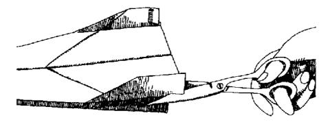
In a real plane there is usually one vertical stabiliser in the tail. The movable flap on the back edge of the stabiliser is called the redder. The rudder works in a way similar to that of the elevators. When the rudder is angled to the left, it pushes against the air. The air pushes back and the tail of the plane swings to the right. When the tail of the plane moves right, the front of the plane moves left. Can you explain what happens when you angle a rudder to the right?
