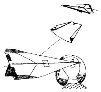
Most real aeroplanes have flaps on their wings and on the horizontal stabilisers in the tail of the plane. The flaps on the wings are used to increase the lift during take-offs and landings, when the plane is moving at its slowest speeds. Remember that the slower the plane moves through the air the less lift it gets. The pilot can vary the angle of the flaps to change the amount of lift.
