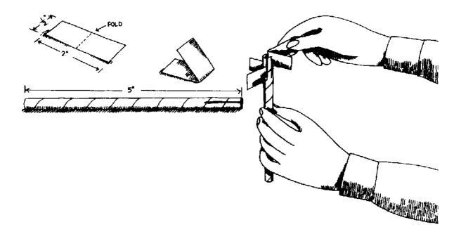
Insert each strip into the end of the straw so that you get four fins at right angles to each other. Throw the straw in the same way as you did before. Compare the way the straw moves through the air with and without the stabilising fins.
