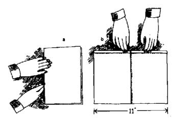
Fold the paper in half crosswise (a). Open the paper and make a crease along one of the long sides, t inch (13 mm) from the edge (b). Make seven to ten more creases in the same way.
