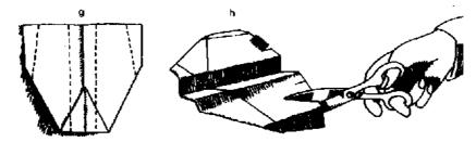
Refold the plane very firmly along the midline. Open the paper. Fold the left wing over along the dotted line shown to the left of the midline in drawing g. Fold the right wing over along the dotted line shown to the right of the midline in drawing g. Turn the plane over (h) and fold each wing tip down, along the domed lines shown in drawing g. Cut small flaps in the back of each wing (h).
