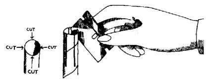
Now cut four one-inch (25-mm) slits at right angles to each other at one end of the straw. From some stiff paper such as an index card, cut two 2-by-0.5-inch (51 mm-by-13 mm) strips. Fold each strip in half-length wise.
