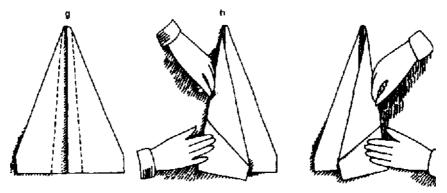
Turn the paper over. Fold one side over (h) along the left-hand dotted line shown in drawing g. Open the paper. Fold the other side over (i) along the right-hand dotted line in drawing g. From the bottom your plane should look like the one in drawing j.
