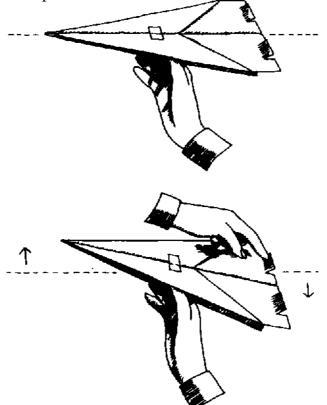
Fold the flaps downwards and again push against them with your fingers. This time the back end of the plane is pushed up. The front end points down and the plane dives.
