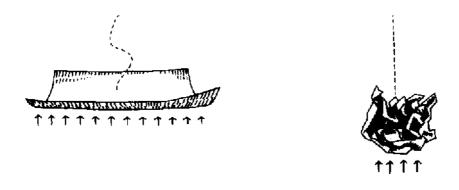
Air is a real substance even though you can't see it. A flat sheet of paper falling downwards pushes against the air in its path. The air pushes back against the paper and slows its fall. A crumpled piece of paper has a smaller surface pushing against the air. The air doesn't push back as strongly as with the flat piece, and the ball of paper falls faster. The spread-out wings of a paper aeroplane keep it from falling quickly down to the ground. We say the wings give a plane lift.
